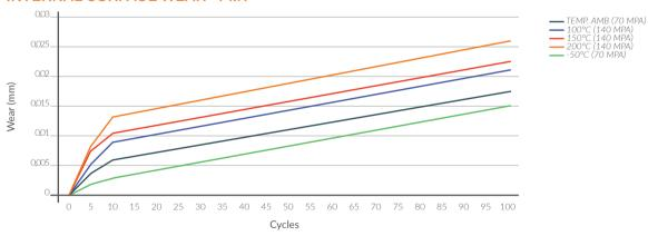
The tests were performed in the Slib Italy laboratory with a Test Bench for the simulation of ball valves
