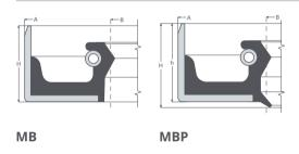
These variations of the G and M type seals are engineered to withstand pressure up to 10 BAR (1 MPa), although this limit has been exceeded in some applications. These seals are available with or without an additional
